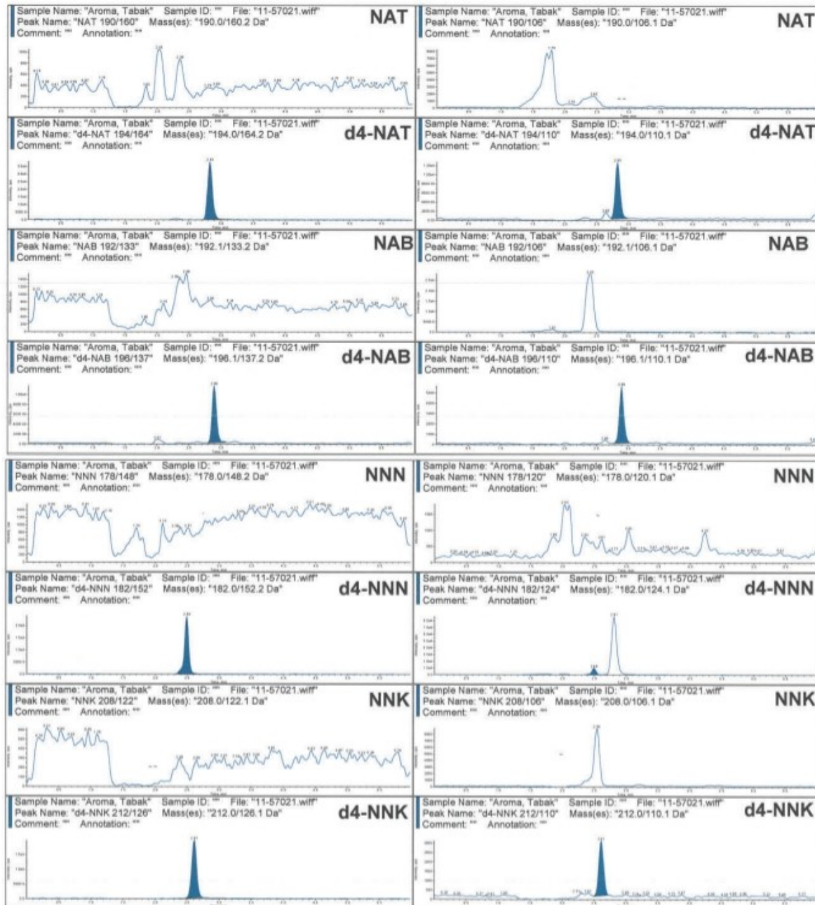
Figure 1: two mass transitions of the isotopically labelled internal standards (added to the sample) and the corresponding TSNAs; the peaks of the isotopically labelled internal standards refer to a concentration of 18 ng/mL sample and 1 ng/mg nicotine (1 ppm), respectively
